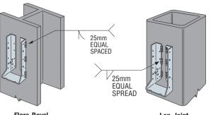
Flare-Bevel **Groove Weld** (See Detail) Lap-Joint Fillet Weld
