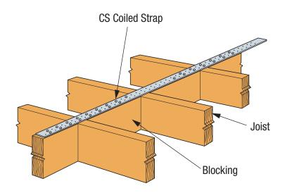
SIMPSON Strong-Tie® CS Horizontal Bracing - Across Joists
