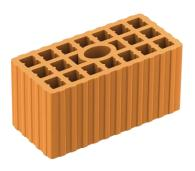
Category c: Hollow masonry: **Doppio UNI (12.12.25)** Bulk density class  $\rho$ =0.9 kg/dm³ Minimum compressive strength fb=6.0 MPa
