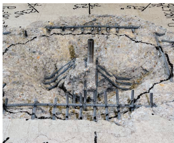
Anchor reinforcement testing at Tye Gilb Laboratory for edge and away-from-edge conditions.
