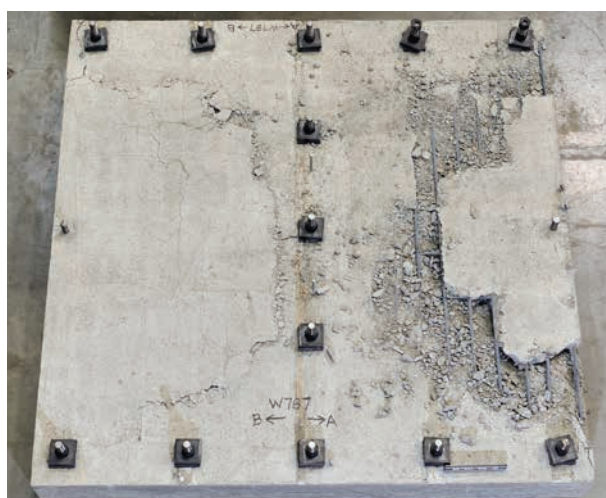
Anchor reinforcement testing at Tye Gilb Laboratory for edge and away-from-edge conditions.
