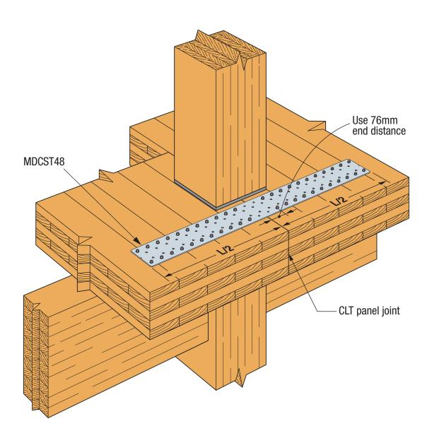
SIMPSON Strong-Tie® MDCST48 Diaphragm Chord Tension Across CLT Panel Joint
