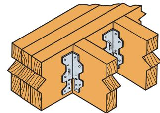
Ceiling Joists to Beam
