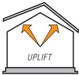
1. **Uplift** – wind flows over the roof of the building, creating a lifting effect.
