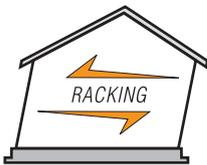
1. **Racking** – earthquake forces can cause the home to move or tilt from side to side.
