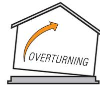
3. **Overturning** – earthquake forces can cause the walls of the home to lift or rotate off the foundation.
