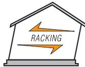
2. **Racking** – wind exerts horizontal pressure which can cause the building to tilt.
