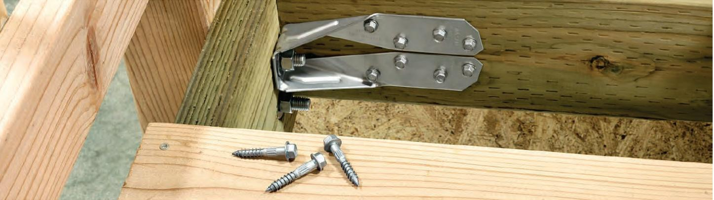
The Simpson Strong-Tie® Strong-Drive® SDS Heavy-Duty Connector screw is a 6.4mm diameter structural timber screw ideal for various connector installations as well as timber-to-timber applications. It installs with no pre-drilling and has been extensively tested in various applications. Available with a double-barrier coating or in Type 316 stainless steel. Carbon steel loads apply to corresponding stainless steel models.
