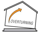
4. **Overtopping** – when the building is unable to rack or slide, wind can cause the walls to rotate off the foundation.
