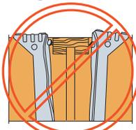
**Toenailing causes squeaks** and improper hanger installations. Do not toenail I-joists before installing top flange or face mount hangers.
