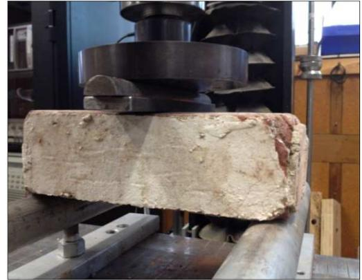
(h) Typical brick rupture test setup
