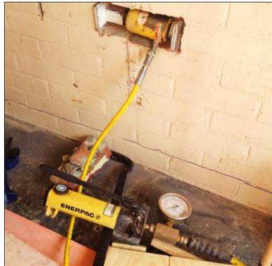
(a) Mortar bed joint shear test setup on Wel-W1
