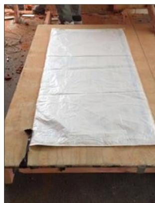
(b) Single vinyl airbag on plywood backing
