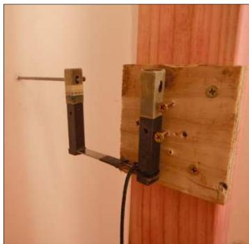
(d) Strain or "portal" gauge spanning between the test wall and the isolated instrumentation frame
