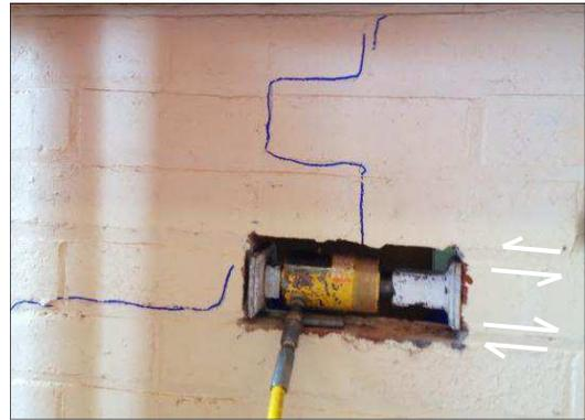
(b) Mortar bed joint shear test setup on Wel-W2 with cracks propagating from load highlighted in blue
