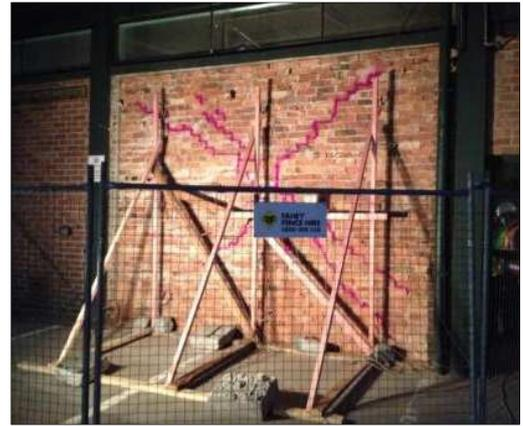
(c) Displacement instrumentation frame for long-wall with cracks from OOP two-way flexure highlighted
