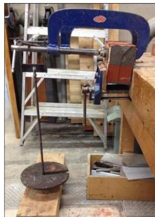
(e) Typical bond rupture test setup
