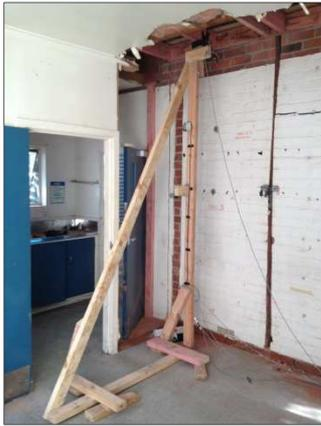
(a) Displacement instrumentation frame for narrow-length wall
