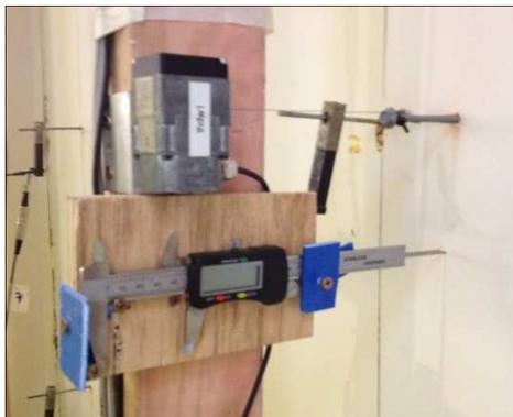
(f) Redundant instruments (portal gauge, string potentiometer, and digital callipers) at the critical centre location on the test wall
