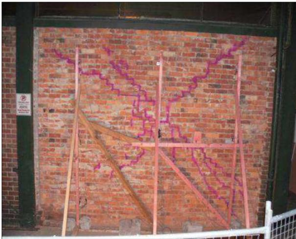
(a) Crack pattern post-loading on the instrumentation side of Auc-W4
