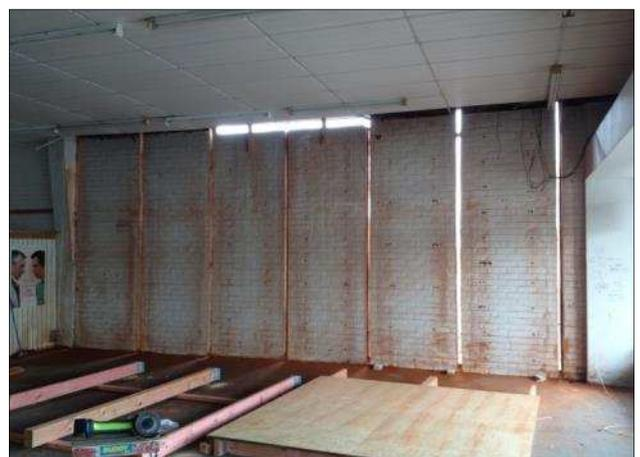
(c) Interior elevation of test walls Has-W1 – Has-W6 (right to left) after saw cutting
