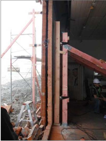
(f) Profile of OOP test bracing (right of wall) and displacement instrumentation frame (left of wall)
