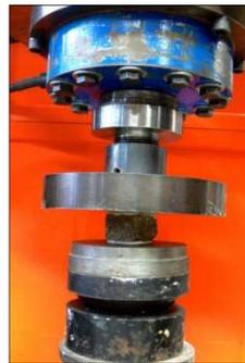
(b) Typical mortar compression test setup
