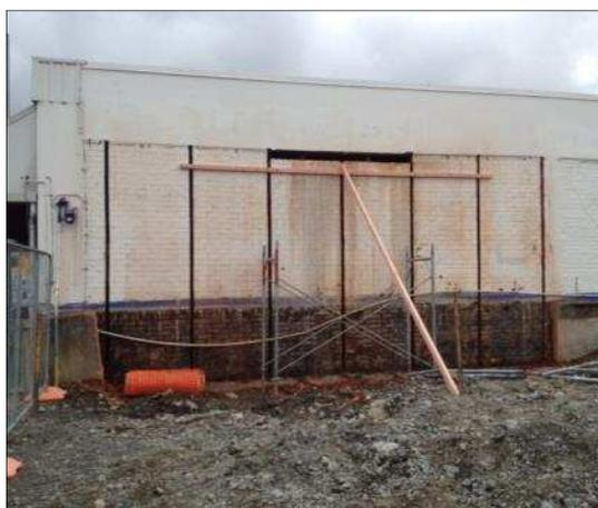
(b) Exterior elevation of test walls Has-W1 – Has-W6 (left to right) after saw cutting
