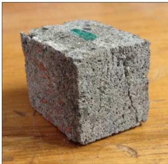
(a) Typical mortar cube cut for testing prior to plaster capping
