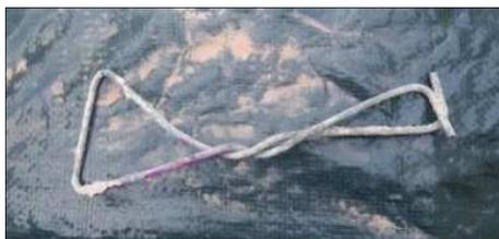
(c) Twisted “figure eight” wire cavity ties
