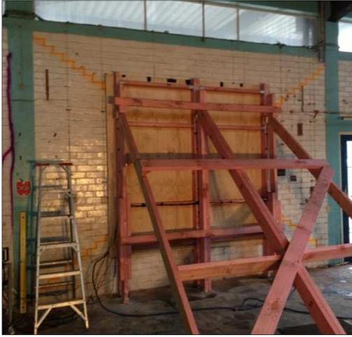
(d) Reaction frame arranged to test one wall panel with two air bags inflated simultaneously
