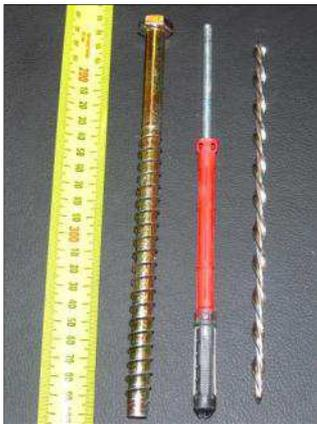
(a) The three retrofit ties used in addition to the in situ ties in Auc-W1B, Auc-W2, and Auc-W3, respectively (left to right)
