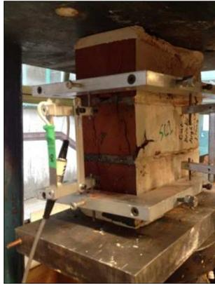
(g) Typical stacked masonry prism compression test setup with four portal gauges used to measure stiffness
