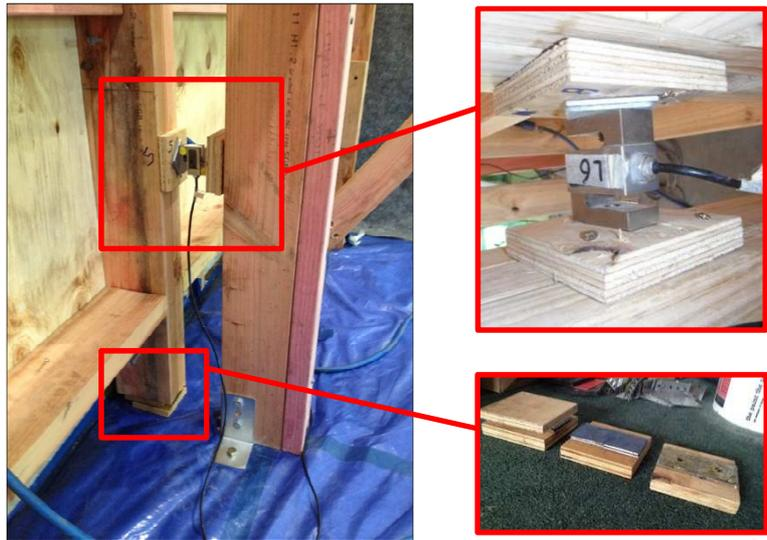
(g) Close-up of base of reaction frame with s-shaped load cell placed between the plywood-backed panel frame and the braced reaction frame (top), and the plywood-backed frame sitting atop greased steel low-friction plates and loose plywood pieces
