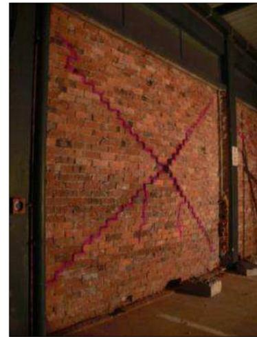
(b) Crack pattern post partial loading on the instrumentation side of Auc-W5
