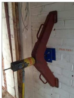
(a) Brace, load cell, and attachment used to pull out cavity tie from brick wall
