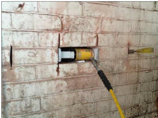
(c) Mortar bed joint shear test setup on Auc-X1 (on otherwise untested wall)
