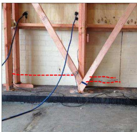
(a) Horizontal crack near the bottom on the loaded side of Wel-W2B (marked for emphasis)
