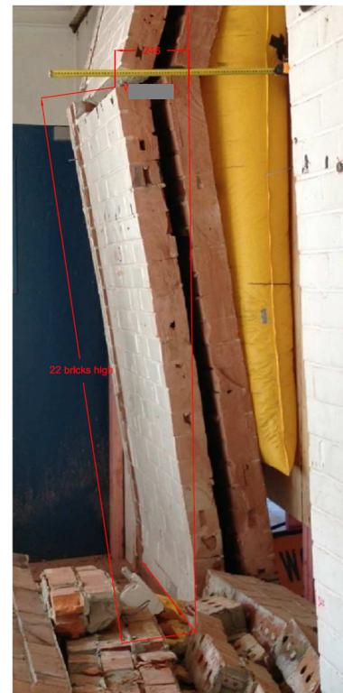
(f) Horizontal crack near five-eighths height on the instrumentation side of Auc-W3 (example of use of photogrammetry to determine instability drift)
