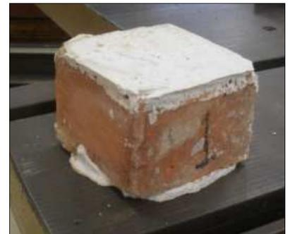
(c) Typical clay brick cut into half-length and capped with plaster for compression testing
