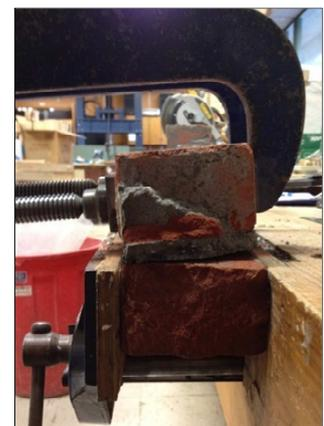
(f) Bond rupture at interface of brick and mortar
