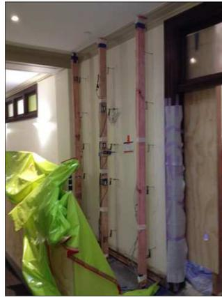
(b) Displacement instrumentation frame for medium-length wall
