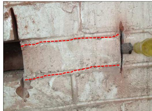
(d) Mortar bed joint shear damage from testing on Auc-X1 (an otherwise untested wall) with shear cracks highlighted in red
