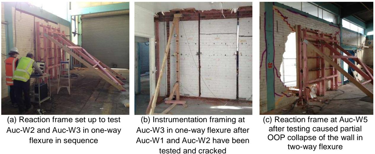
**Figure 22:** Examples of the test setup and instrumentation at the Auckland building
