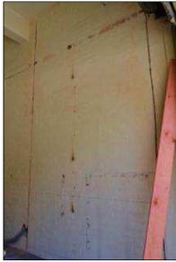
(a) Loaded side of Wel-W1 with vertical saw cuts
