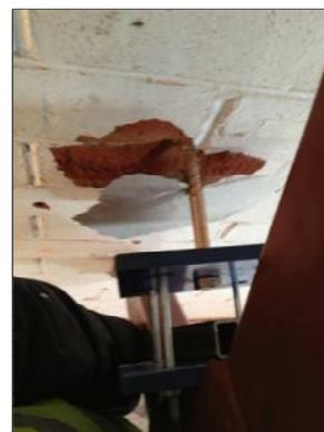
(b) Pull-out failure due to brick conical shear
