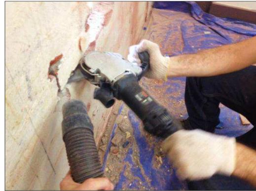
(b) Dry saw used to extend vertical cuts through wall and extract bricks for bed joint shear testing
