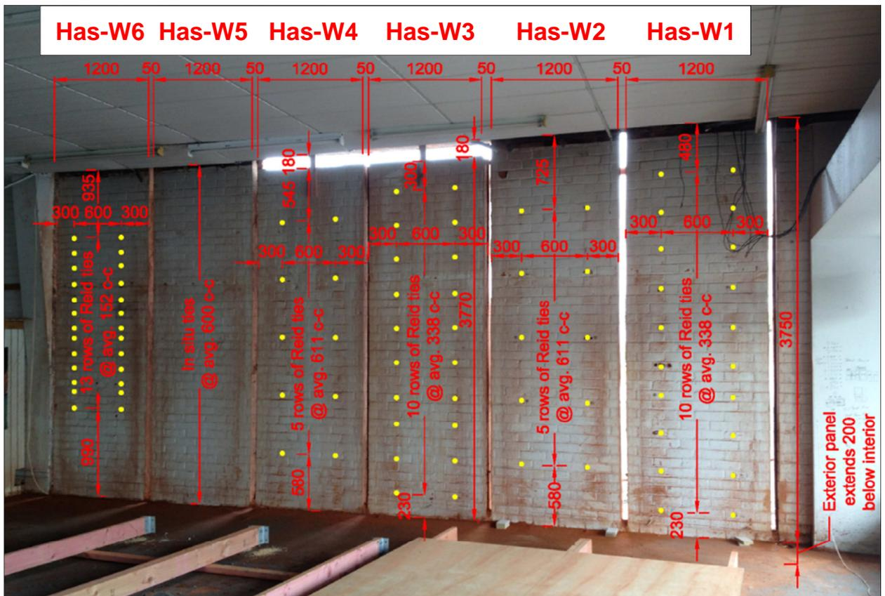
**Figure 9:** Dimensions of test walls at the Hastings building and spacing of mechanical cavity ties
