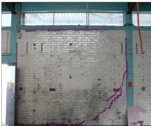
(c) Crack pattern post-loading on the loading side of Auc-W4
