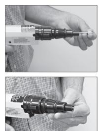
Insert the fastener into the nosepiece of the tool, head or threaded end first. Push the fastener until the pointed end is even with the face of the nosepiece, or if a pre assembled fastener is used, until the nose piece is against the fastener accessory.
