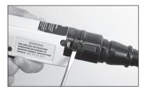
1. Rotate the annular spring off the piston stop with a flat blade screw driver or long fastener.
