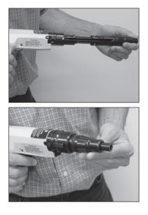
Open the tool. Grasp the nosepiece and pull sharply forward until you feel a positive stop, then pull the nosepiece back until it stops and is fully closed. This resets the piston and positions the advance lever in the correct location for inserting the strip loads.
