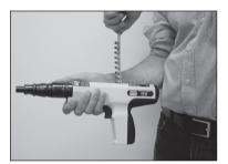
Remove the spent powder strip load by grasping the strip from the top side of the tool and firmly pull upwards in a smooth motion.
