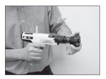
5. After making the fastening, lift the tool off the work surface and pull the nosepiece sharply forward, or flip the tool open with a snap of the wrist. This action resets the piston and advances the powder load strip to the next powder load.
